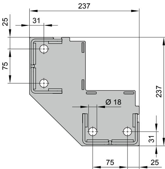
07 72282. Post bracket for fixture to the markant
